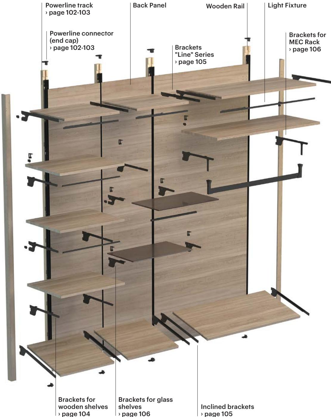
NOTE: Powerline System does not include shelving material, i.e. wood or glass.
